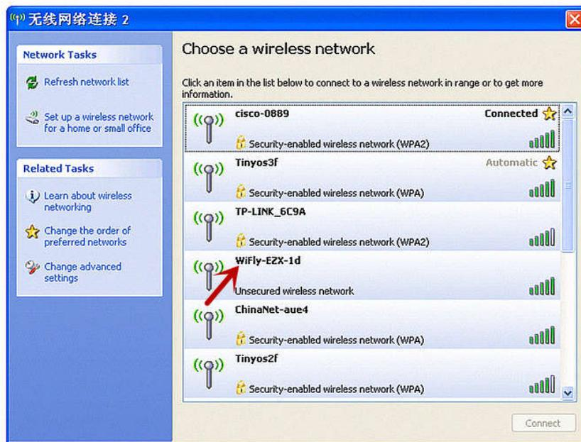
**NOTE:** It may take a while for Windows to connect to the network and assign an IP address. You can check the IP address of your computer by running the ipconfig command in the command window. Once connected, this command will show you the IP address and net mask.
