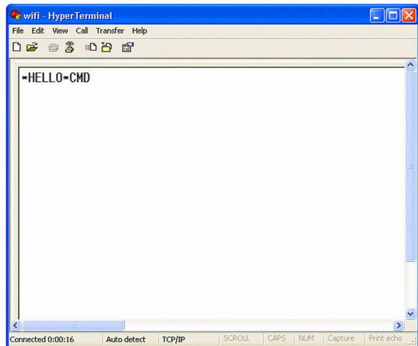
(5) Now you can setup WiFi module's settings. Input every command on your keyboard, and click the **Enter** button after each command to send. The Hyper Terminal should return **AOK**.
